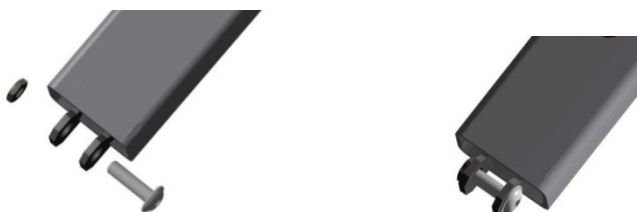
Figure 4: Insertion of the new connection components
