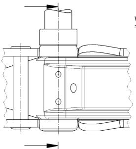
Weld seam execution according to DIN EN ISO 13920-BF >UTP 8 is recommended as welding rod electrode for the cold welding
