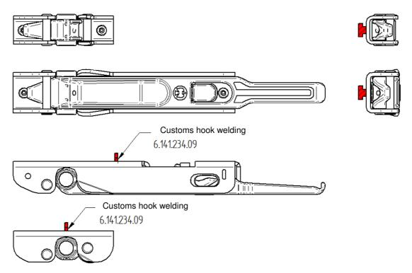
As a rule, two locks per door leaf are fitted by the customer for double rear doors, i.e. a total of 4. For doors with centre overlapping door rabbets, the lock in the centre of the customs model vehicle is intended for the out-lying door, meaning only one of the total four locks.
