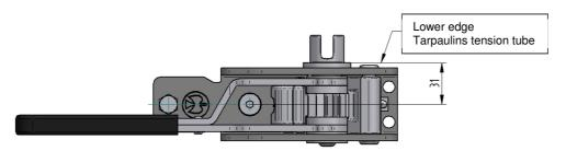
The HESTAL *TensionMaster IV* is bolted to the outer frame as follows:
